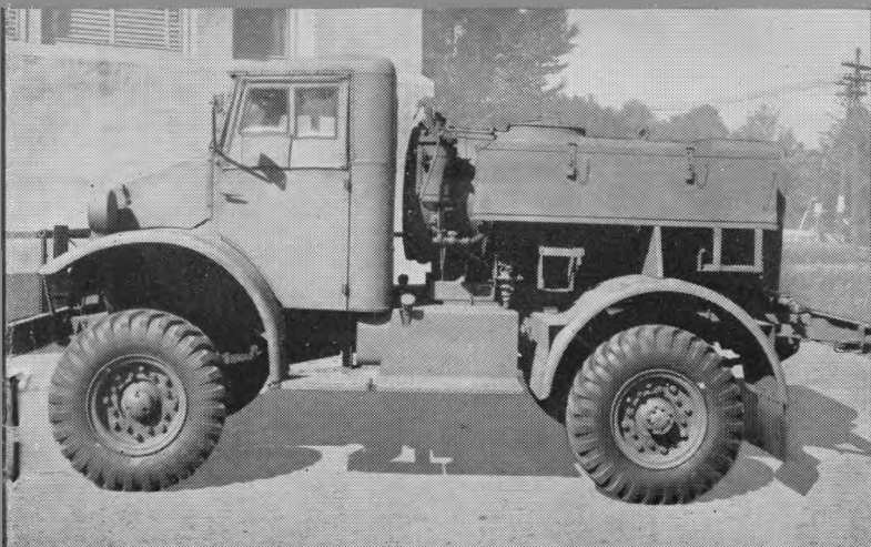
WATER TANK PURIFIER TRUCK —Marching men need water and to assure a constant supply, tank trucks like this transport it. Built into the body is a chemical purifier which renders all water drinkable.
